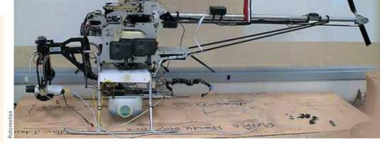
Shorn of its fairing, a UAV is a serious piece of complex avionics.
